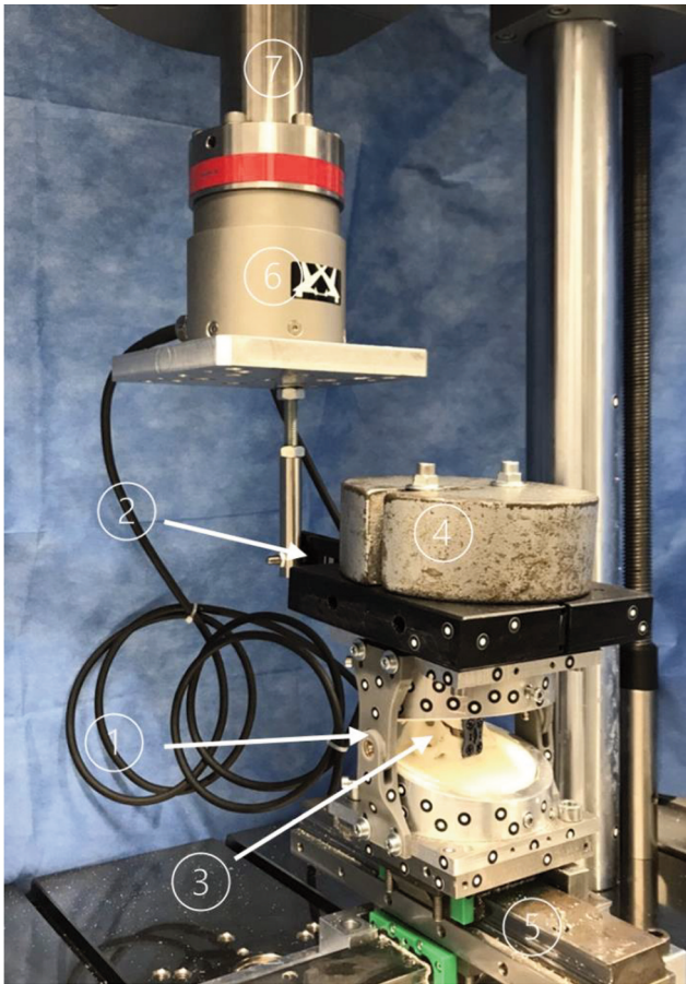
Figure 4. Test set-up. 1) 3D-printed supports with a central ball bearings-joint against rotational shear forces, 2) telescoping rail as lever arm, 3) specimen, 4) initial load of 50 N, 5 x-y-table, 6) load cell, 7) testing machine.
