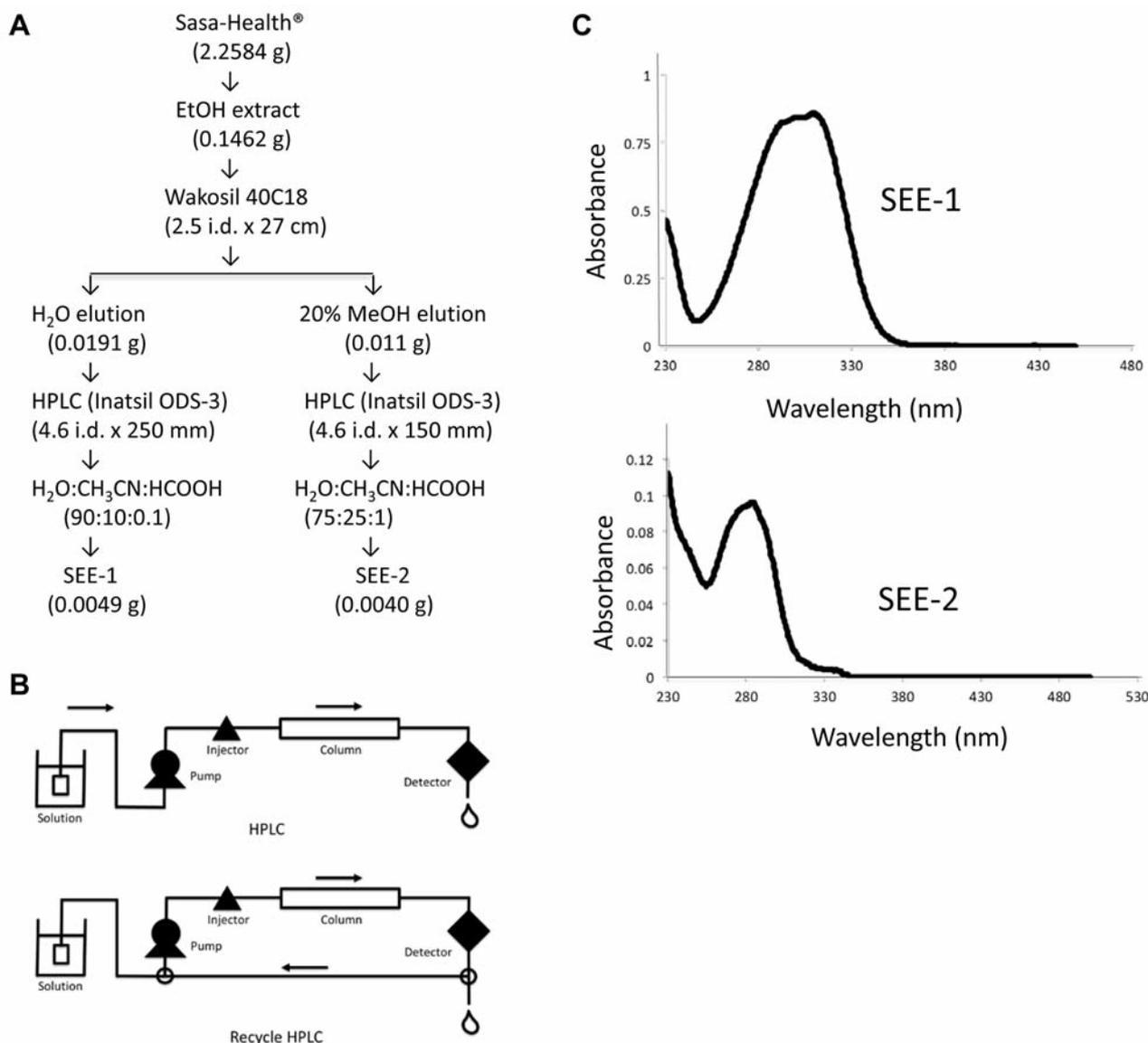
Figure 1. Isolation of SEE-1 from Sasa-Health®. A: Procedure for purification of SEE-1 and SEE-2, using recycle HPLC (B). C: UV absorption spectra of SEE-1 and SEE-2.
