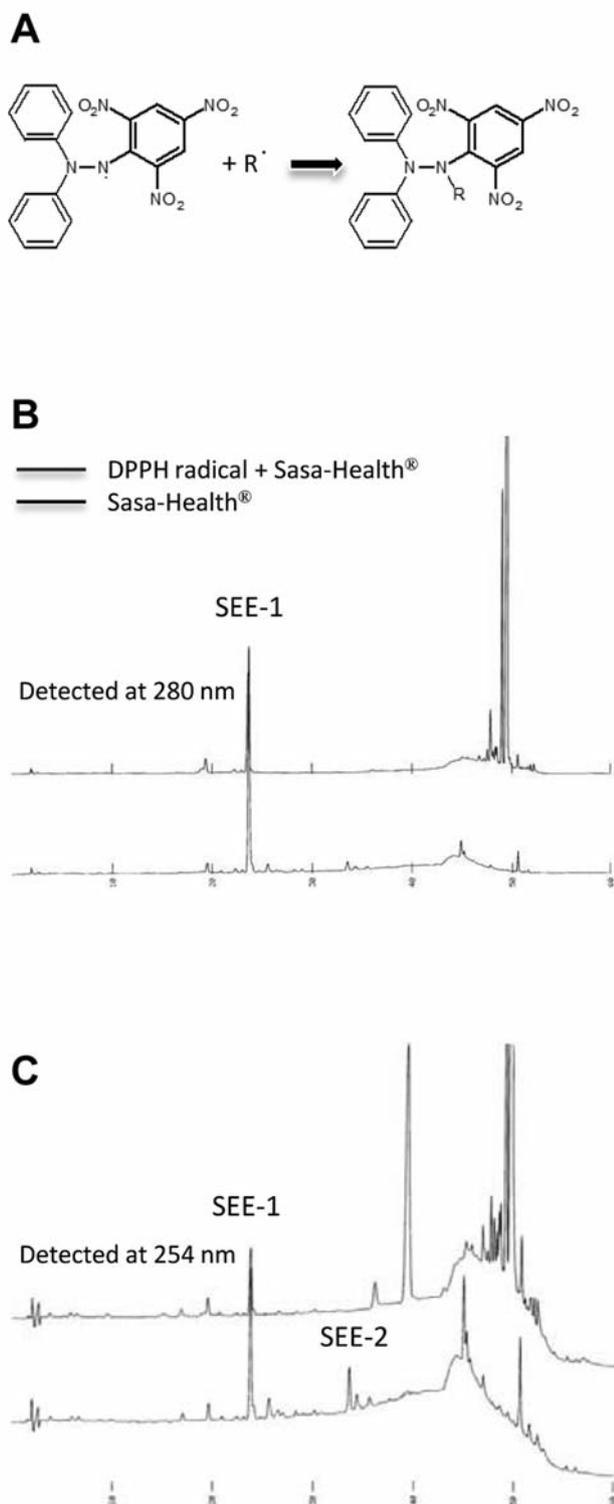
Figure 4. 1,1-Diphenyl-2-picrylhydrazyl (DPPH) radical-scavenging activity of Sasa-Health<sup>®</sup> by HPLC analysis. A: Reaction scheme of DPPH radical and anti-UV substance (indicated by  $\bullet R$ ). B and C: Elution profile of Sasa-Health<sup>®</sup> alone (lower) and with DPPH radical (upper) on HPLC (Inertsil ODS-3) fraction, detected at 280 nm for SEE-1 (B) and 254 nm for SEE-2 (C).
