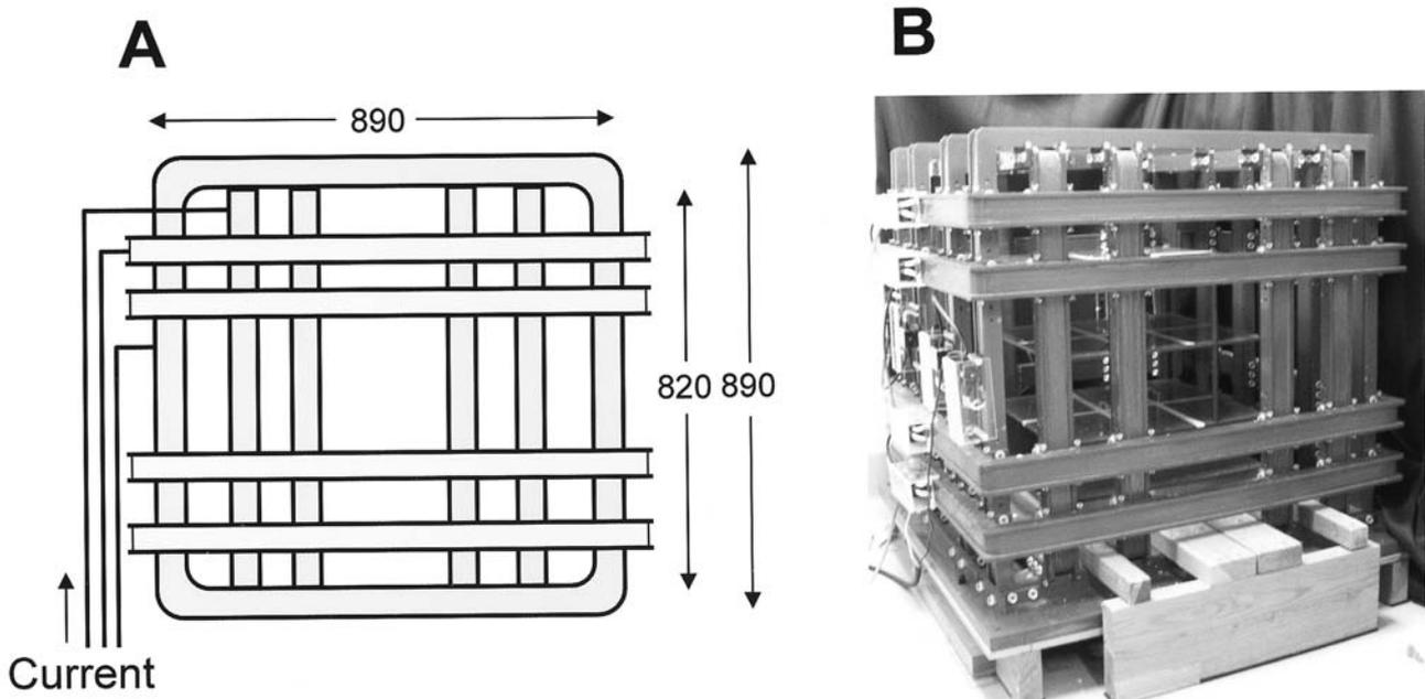
Figure 3. Design of ELF-EMF generating coils. (A) Front view of Helmholtz coil. Coils were connected to the power supply and the current in each coil was regulated independently. Unit of numeral in figure is mm. (B) Photograph of the exposure set-up. The animal rack is located at the center of coils, and is separated from the coils to prevent vibration.
